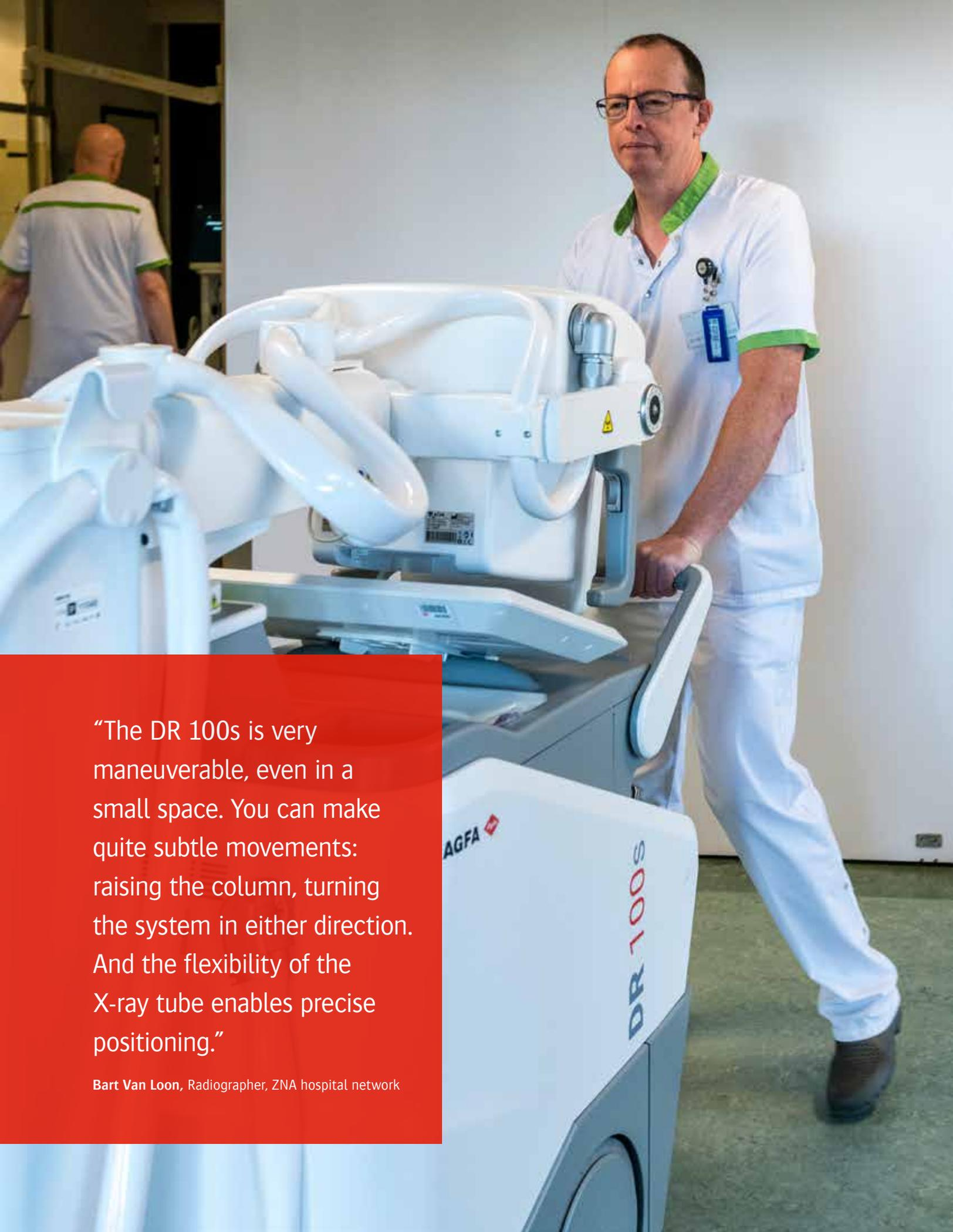
“The DR 100s is very maneuverable, even in a small space. You can make quite subtle movements: raising the column, turning the system in either direction. And the flexibility of the X-ray tube enables precise positioning.”
